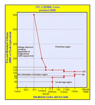
The ITIC (CBEMA) curve describes several ranges for voltage variation events. The voltage variation can be plotted on the graph as a point. The magnitude of the event as referenced to the nominal voltage is the X coordinate and the duration of the event in either cycles or seconds is the Y coordinate. Once the point is plotted it is easy to see if the event could be the cause of information technology equipment malfunction. (Computers, Faxes, routers, modems, internet, televisions...etc.)
